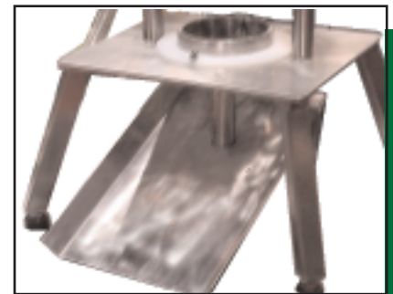
Divider pan separates product from core
