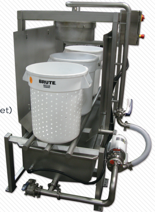
*Open design, Three Stations: On deck, Wash, Drain
