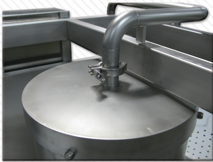
*Shower head disassembles for easy cleaning
