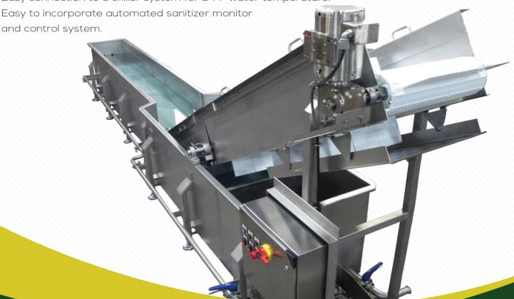
The Melon Washer is designed to sanitze melons prior to peeling. The melons are loaded in the feed end of the washer and the jets push it to the exit conveyor. The pump speed is variable to accommodate various sized melons and dwell time. An automated sanitizer monitor and control system can be easily added to the wash system. Other confirgurations are available to meet the specific needs of each processor.
