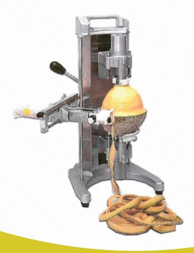
The versatile, easy to use CP-44 fruit peeler is the perfect system for peeling all kinds of round fruit - melons, avoca-dos, mangos and more. The peel depth is easily set by the operator, and follows the contour of the fruit for maximum finished product yield. Peeled product output is approximately six melons per minute. The system is easy to clean and store - with a footprint of only 11 x 17 inches.
