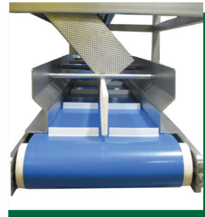
Cores are discharged on left side and good slices on the right side
