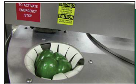
Peppers are placed in carousel pockets and indexed to the cutting position.
