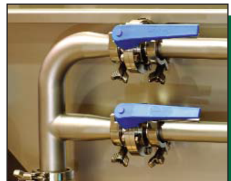
Sanitary valves and manifold fittings
